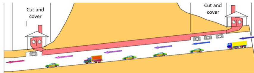
**Figure 10: Layout of the 3<sup>rd</sup> Gubrist tunnel tube.**
