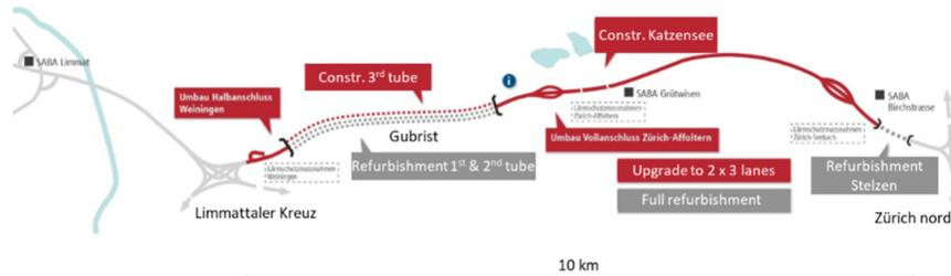
**Figure 1: Overview of the ongoing works on the NRRZ (Source: FEDRO).**
