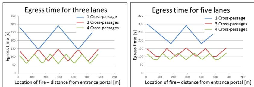
Figure 8: Total egress times as a function of fire location.
