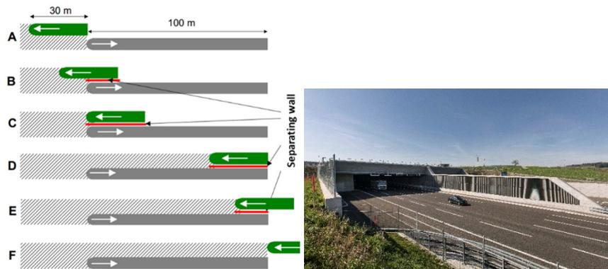
**Figure 3: General principles of prevention of smoke recirculation at portals (1) and implementation in tunnel Katzensee (Source: FEDRO).**
