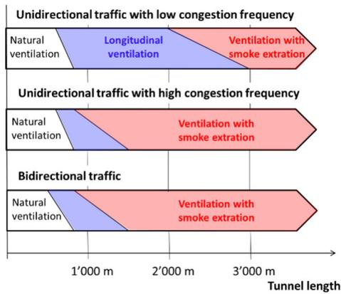
**Figure 2: Selection of ventilation system according to ASTRA 13001.**
