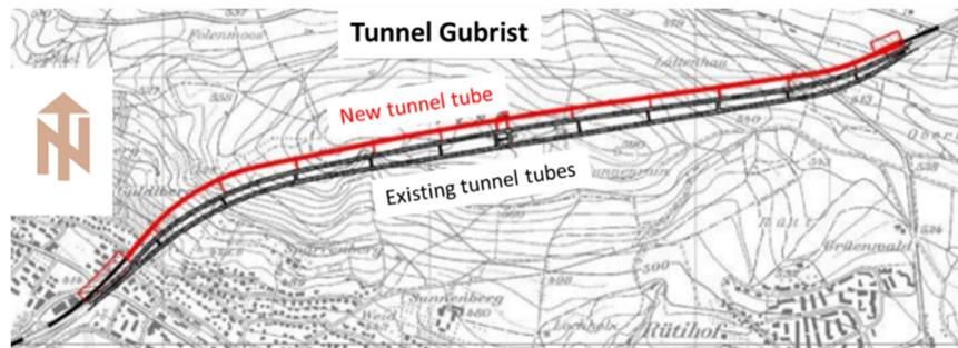
**Figure 9: The 3 Gubrist tunnel tubes (3<sup>rd</sup> tube in red).**
