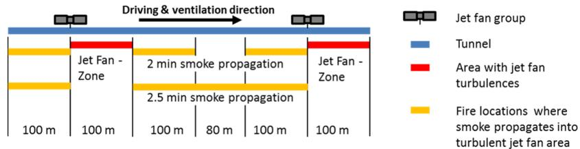
**Figure 7: Illustration of fire locations where activation of jet fans would result in destratified smoke propagation for fan installation in the tunnel.**
