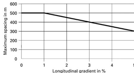
**Figure 4: Maximum spacing of emergency escape routes for mined tunnels according to SIA 197/2.**
