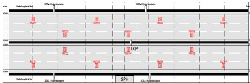
Figure 5: Location of smoke sensors in tunnel Stelzen.
