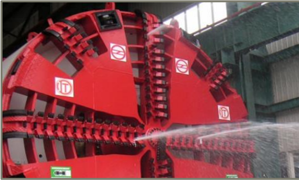
■ View of drilling head of the EPB-TBM
