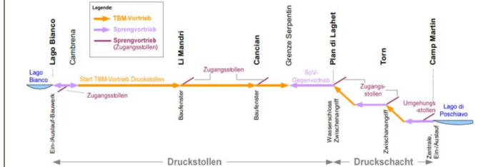
Schedule advancing headrace gallery and shaft
